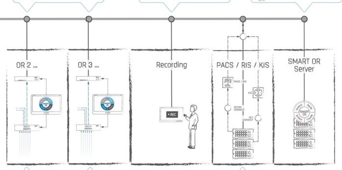
You can create separate user profiles for every OR, meaning you can create profiles specifically tailored to a procedure, a room or a user. Prepared worklists are transferred and displayed in the OR. Images and findings collected during treatment can be linked to the information in PACS and viewed there
